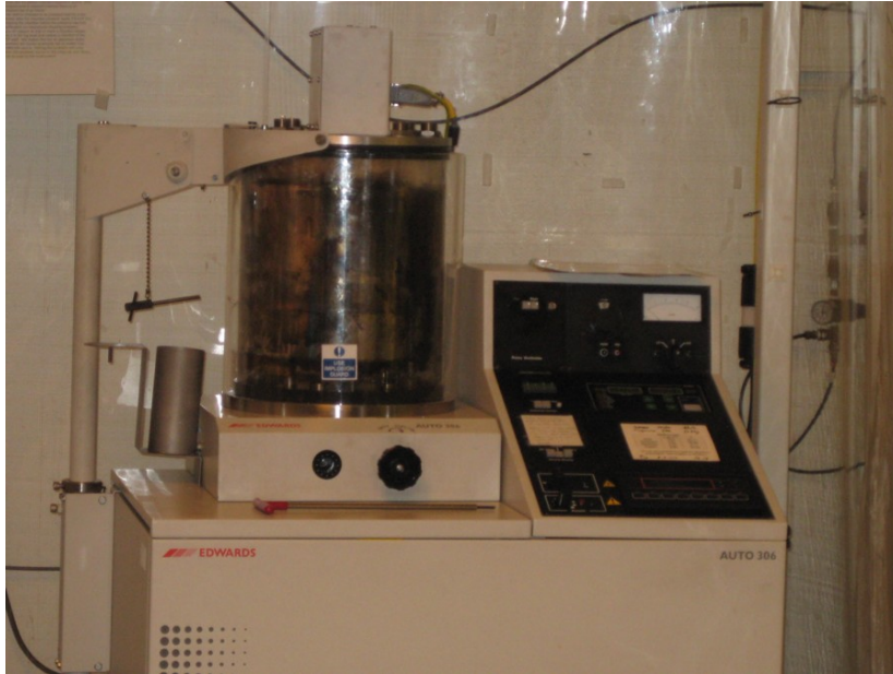
FIG. 2. Thermal evaporator at MCF.
